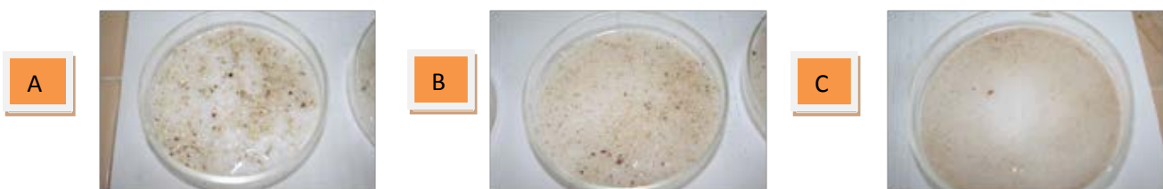
Fig 12. Different samples of flour in water : A : coarse, B : medium, C : fine flour
